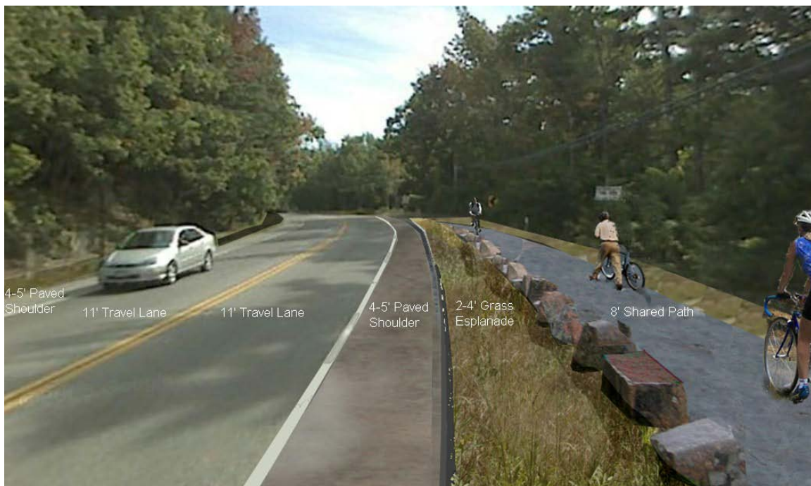
Figure 6 Conceptual Illustration of Sidewalk, Esplanade and Shoulders on Hill to Park Entrance
