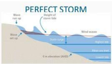
Figure 5-3 Components of storm tide and breaking wave processes.
