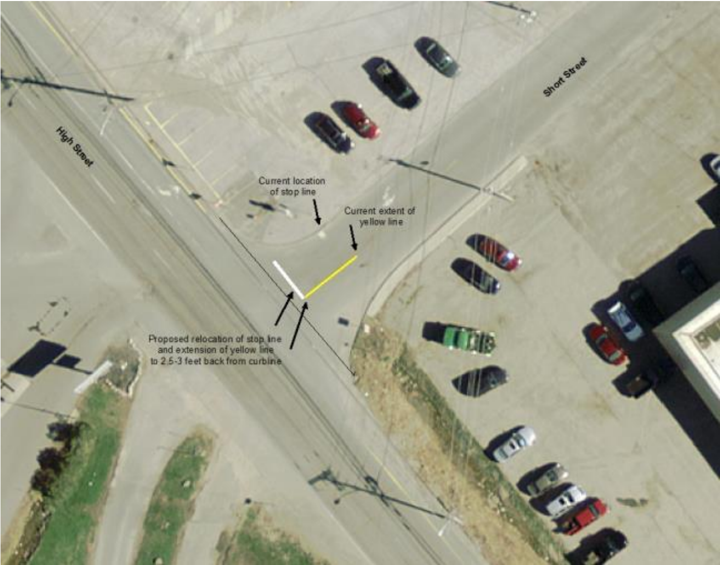
Photo F. Relocate the stop line and extend the yellow line on Short Street.
